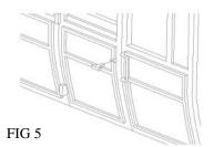
6. You can now solder the door handles and grab rails in place or leave them until after painting - when they will have to be glued. The door handle locating holes may need to be opened out. File the outer edge of the handles to a smooth finish. (Figure 5, above).
